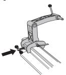
Mount the power cutter with its right side to the fixture.
